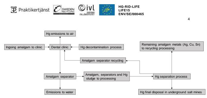
Figure A Schematic picture over the technical system for Hg separation at dental clinics in Sweden.
