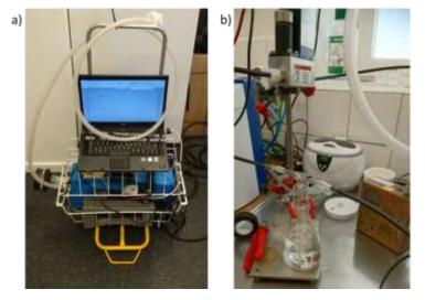
Figure 2 a) Lumex RA-915+ mercury analyzer with computer for data logging. b) Glass bottle with bubbler to measure dissolved gaseous elemental mercury in water samples.
