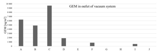
Figure 7 Average GEM concentrations measured at the outlet of the vacuum system, at dental clinic A, B, C, D, F and I, before decontamination.
