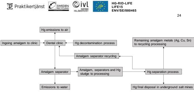
Figure 1 Schematic figure over the technical system for Hg separation at dental clinics in Sweden.
