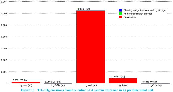
Figure 13 Total Hg emissions from the entire LCA system expressed in kg per functional unit. The functional unit is one dentist's chair for one year of operation (226 working days). Scenario 1: with Hg decontamination, Hg processing, and final Hg storage.
