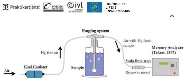
Figure 4 Principle of purging gaseous Hg(0), or DGM, in water samples for analysis. A Lumex RA-915+ mercury analyzer was used for analysis (not a Tekran 2537 as shown in this picture) (Nerentorp Mastromonaco, 2016).
